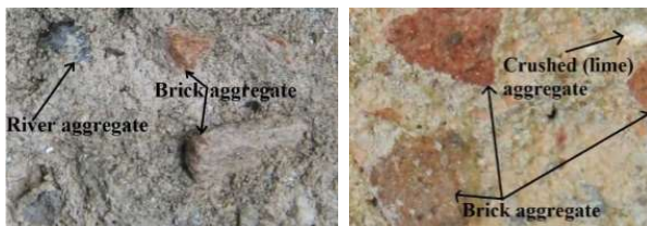
Fig. 12 - Sample detail 5CG (left) and sample flat section surface detail 5CG (right)
