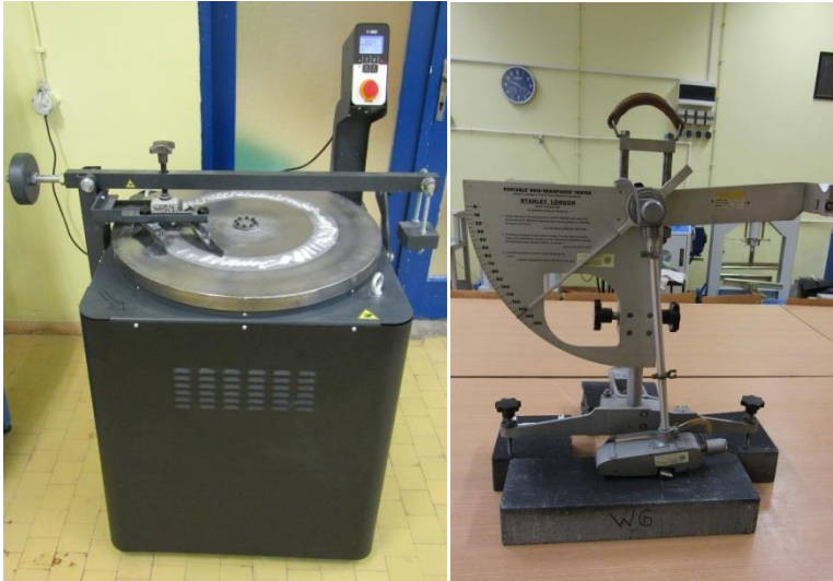
Figure 7 – Abrasion wear test on the Bohme machine (left); Testing of skid resistance by pendulum friction tester (right)
