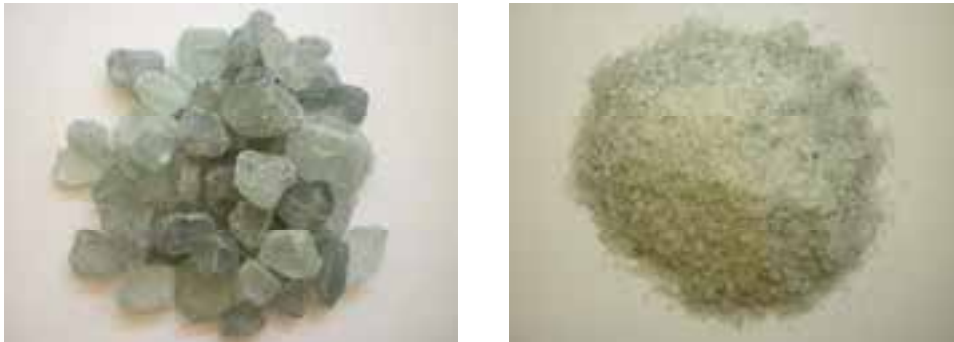
Figure 1. Coarse crushed glass (left) and recycled glass 0/4 mm (right)
