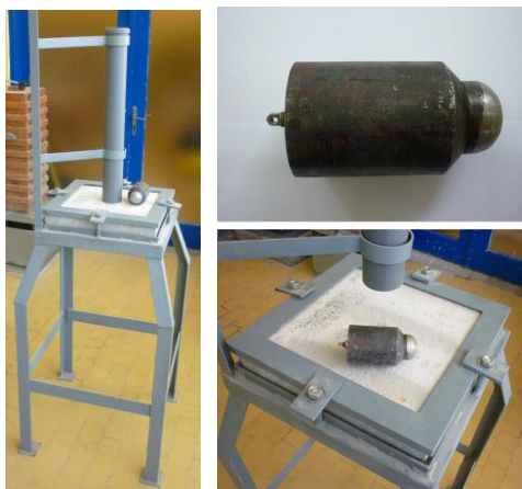
Figure 1 – Test setup of concrete impact resistance testing by the „Drop-weight“ method
