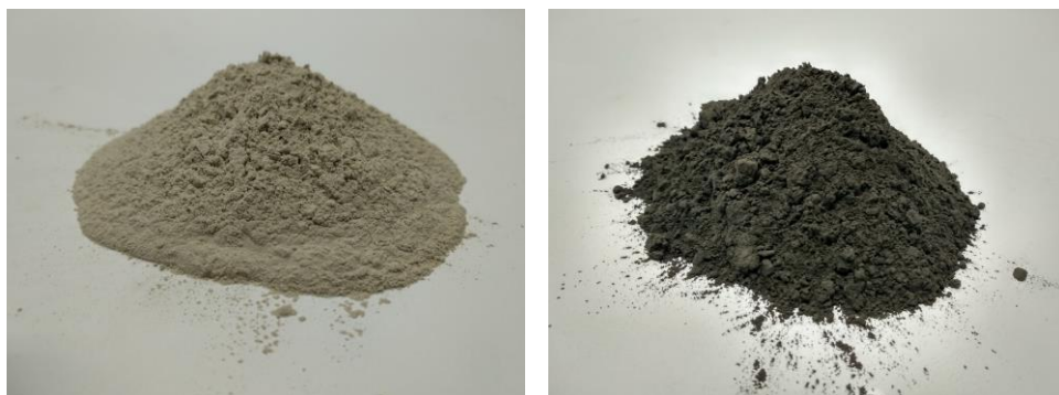
Figure 1 – Used binders: ground granulated blast furnace slag (left) and fly ash (right)
