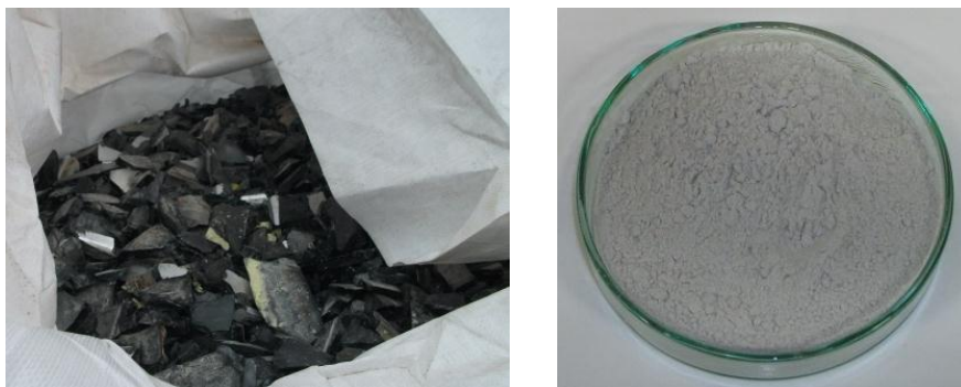
Figure 1 – Glass shards after recycling (left) and milled glass, finer than 0,063 mm (right)
