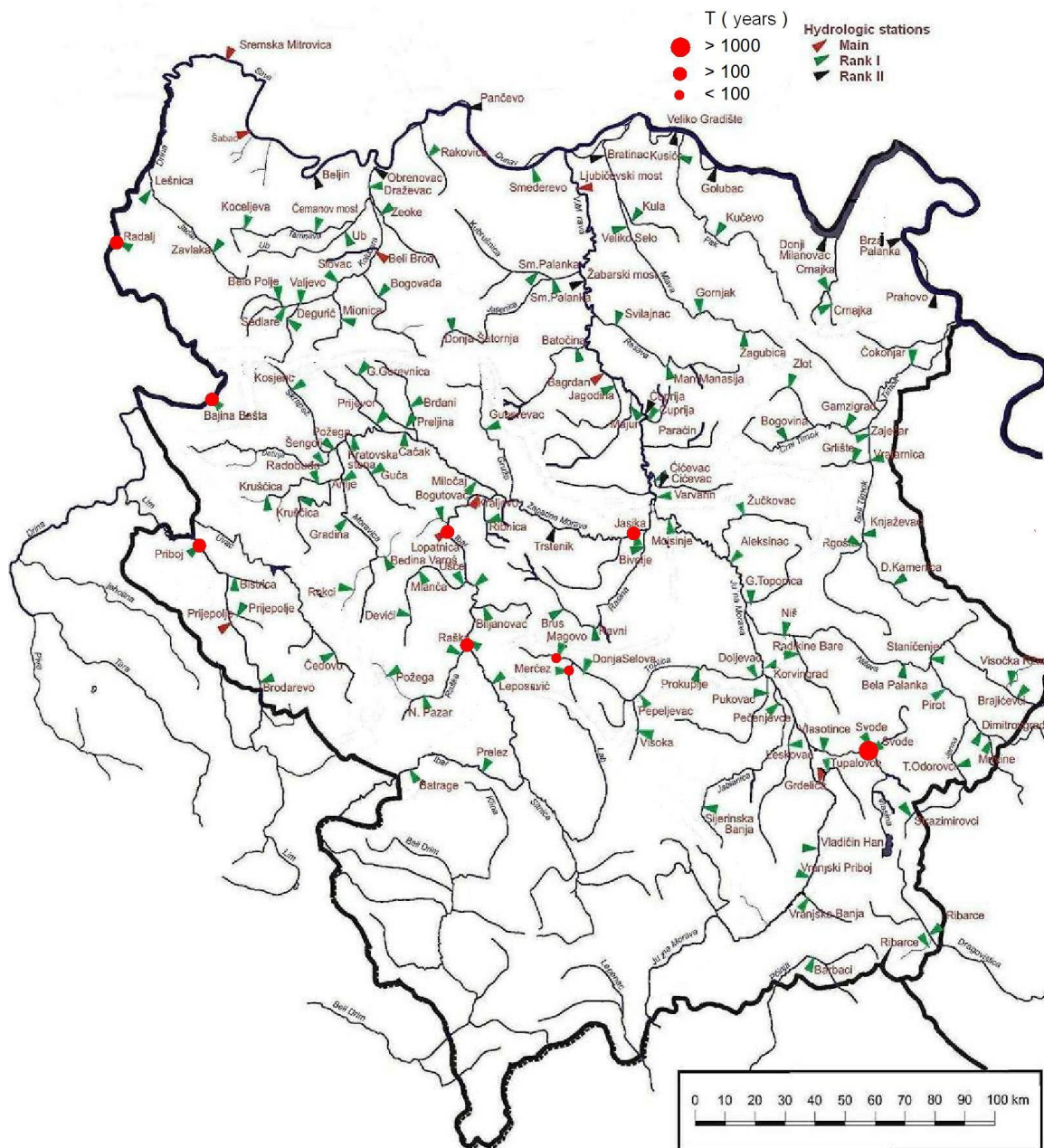
Figure 3 Detected high outliers in AMS data records until 2006 with symbolic representation of estimated return periods (Modified from: Blagojević et al., 2010).
