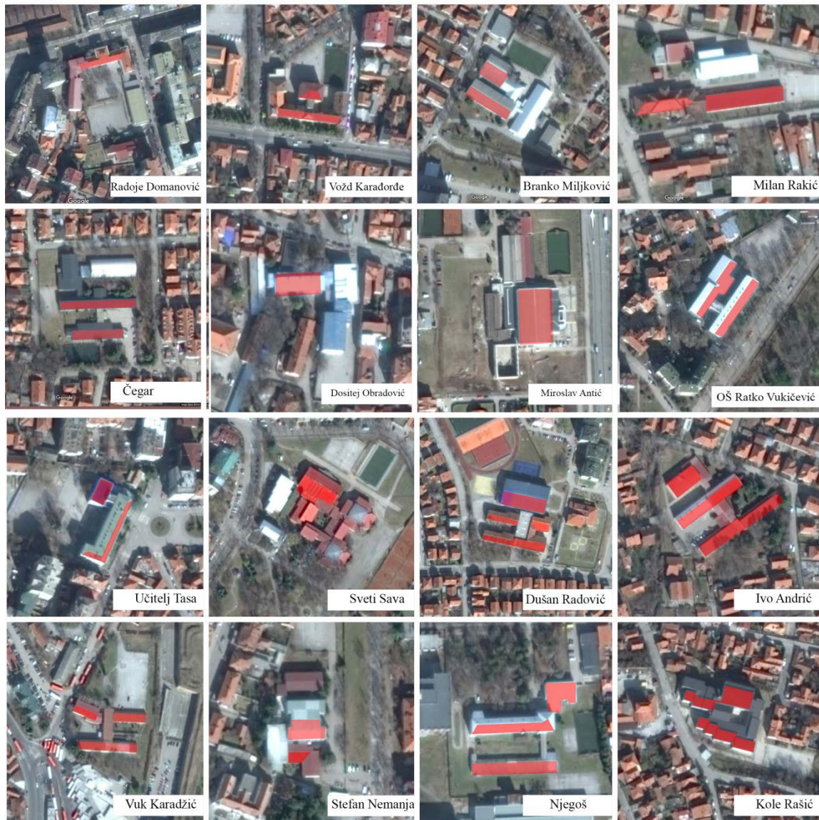
Figure 4: Analysis of possibilities for setting up photovoltaic panels on the roofs of primary schools
