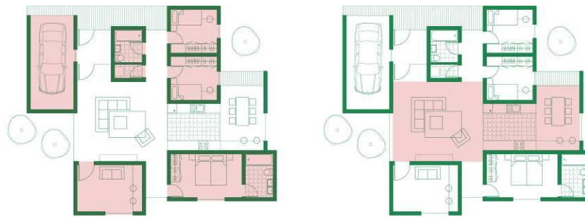
Figure 9 – a) Parents' room divided from children's rooms; garage, workroom and auxiliary facilities inside the separated structures; b) "In between" space as "public" space inside the house
