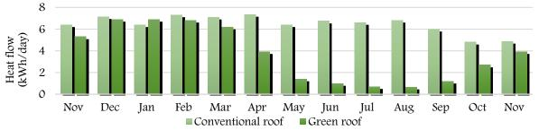
Figure 1. Average Daily Heat Flow through Green Roof and Conventional Roof Systems<sup>3</sup>
