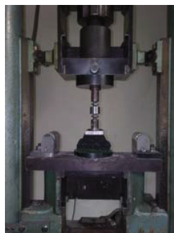
Figure 7: Measuring place for testing of maximum breaking load
