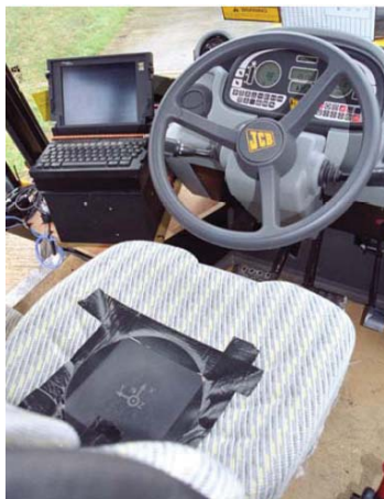
Figure 5. Tractor wbv measurement instrumentation
