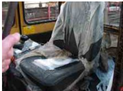
Fig.8. 'Seat' accelerometer configuration incorporating operator presence switch
